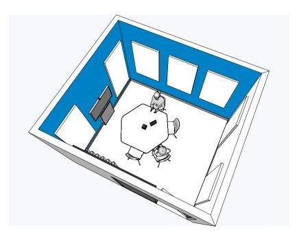
Acoustic treatment on wall areas should ideally feature on two adjacent walls to reduce the risk of parallel reflections forming between two opposite reflective surfaces.
