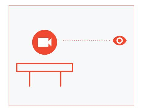
Mount the camera as close to seated eye level as possible. With both screen and camera needing to be central, a compromise is inevitable. Where the camera is placed on top of the screen the bottom of the screen should be 800mm from the floor.
