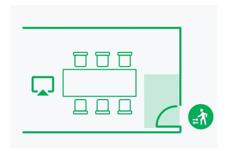
Consider how you might arrive into the space before and during meetings. A well placed entry point opposite the screen wall and away from the table will minimise disruption. Maneuvering clearance is also required at the doorway as per local code and specified by architect.
