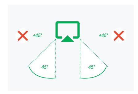
Horizontal viewing angles to video displays should not exceed 45 degrees, measured from the perpendicular of the outer screen edge.
