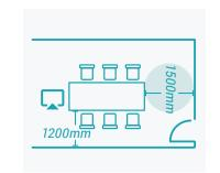
Don't forget the clearance needed between the walls and the furniture for access and wheelchair turning space.
