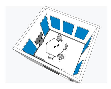
Wall treatment should ideally be placed at seating head height approximately 1m from the floor, up to the ceiling.
