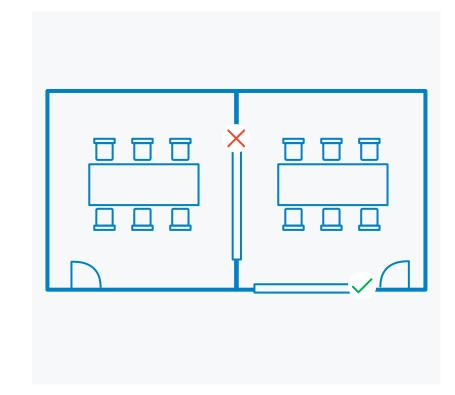
Use of glazing is great for open plan office spaces, but be warned of its inferior acoustic compared to plasterboard walls. Aim to limit glazing to the wall with the entry door, and avoid placing glazings between meeting rooms.
