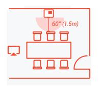
This is the recommended space around the Jamboard to allow effective collaboration. The smallest recommended zone is a semi circle of radius 60" (1.5m) in front of the Jamboard.
