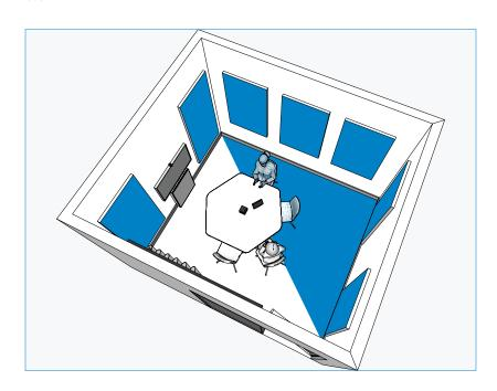
The total area of acoustic wall treatment needed should at minimum be equal to 50% of the total floor area of the room, plus an additional 5m<sup>2</sup> using treatment with an NRC of at least 0.7.
