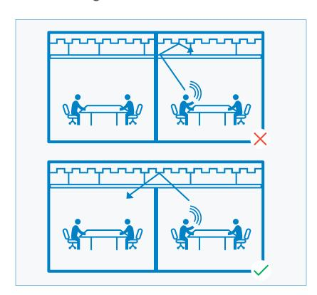
Partitions should be full height. Half height partitions allow for sound to transfer over the wall and limit sound isolation.
