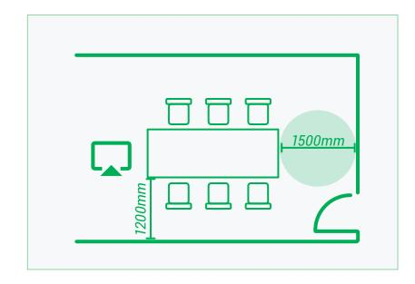
Ensure there is at least 1200mm clearance around fixed furniture for accessibility, this is greater than most local codes to provide good accessibility. A turning circle of at least 1500mm must also be provided between the table and the rear wall.
