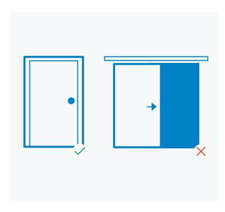
Doors are generally the acoustic weak link as sound is able to go through and flank around the door through the gaps in the doorway. Insulated metal doors are preferred, followed by solid wood doors. Generally swing doors perform better than sliding doors. Perimeter acoustic seals will aid the sound separation performance and should be considered for any meeting room.
