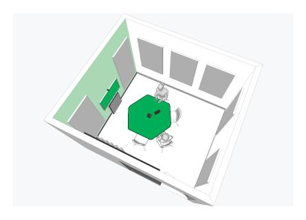
Typically the most efficient use of space is to orient the room 'lengthways' with the screen wall on the short side of the room. The screen wall is ideally a flat, even surface.
