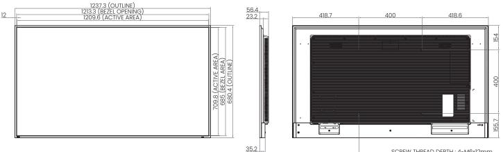
SCREW THREAD DEPTH : 4-M6x12mm
