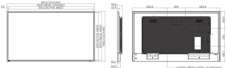
SCREW THREAD DEPTH : 4-M6x12mm
